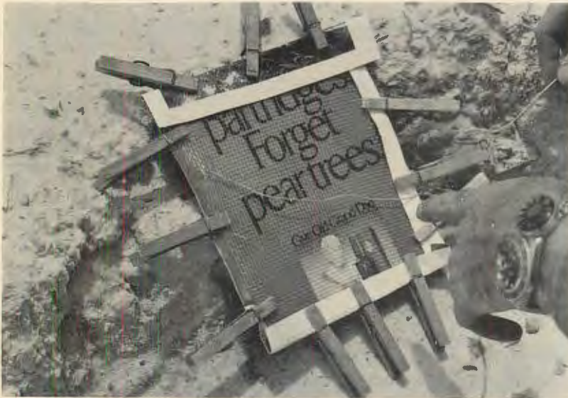
Close-up showing remote "sandwich" with stiff paper separating metal screens and held in place by spring-type clothes pins. Ladas' finger points to wires connecting both screens into firing circuit.
