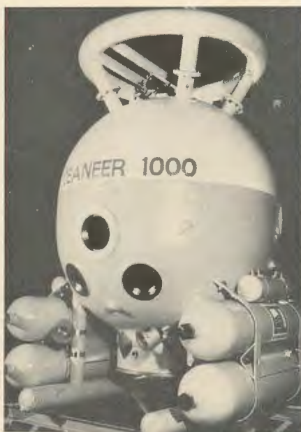
The OCEANEER 1000, designed and developed by Oceaneering International, Inc., the world's largest diving company. Divers exit through the base hatch.
