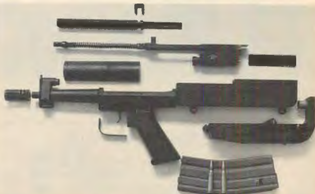
The Bushmaster stripped. Note M-16 parts, such as flash hider, selector button, magazine, etc. The flash hider, however, is comparatively ineffective on the Bushmaster because of the .223 cartridge's "fireball" effect in the short barrel. (The powder grains do not ignite until they have left the tube).
