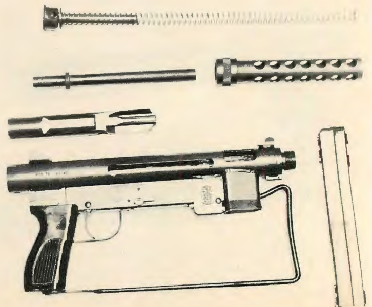
Right: the M76 stripped down to its basic components
