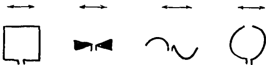
Fig. 5 — Different shaped antennas generate the same linear polarization.
