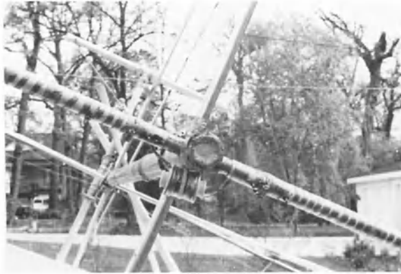
Fig. 7 -- Typical hub. Note the loading coil tuned reflector helix.
