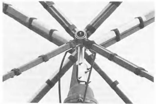
Fig. 11 — An end view of the quad shows pre-cut spreaders against the hub. The hub and axle pipe are self-aligning. The quad is symmetrical with low rotational inertia and presents modest loads to the rotator. Coaxial cable was brought up over the mast T for strain relief. A 7 foot 2 x 2 stiffener was fastened to each upper spreader with shipping tape overwrapped with black vinyl tape for protection from the sunlight.
